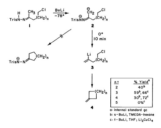
cycloheptane from 30% to 72%, and also marginally increased the yield in 6-membered ring formation as well. The yield of methylene cyclopentane was low due to volatility problems (see below for another example of efficient cyclopentane formation), but the 8-membered ring yield not unexpectedly was essentially nil, even with copper catalysis.
